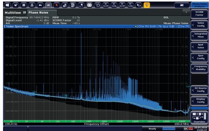
PCIe clock with SSC: phase noise.
