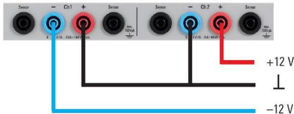
The circuitry of each single channel is completely isolated from the others; there is no connection to chassis ground. This makes it easy to combine the channels to drive balanced circuitries that might need +12 V/-12 V, for example, and avoids ground problems in complex DUTs.
